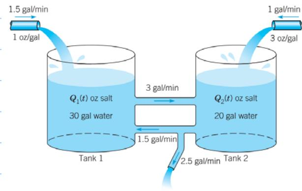
FIGURE 7.1.6 Two interconnected tanks (Problem 19).
