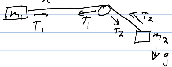
Note:  $T_1$  on pulley is (+),  $T_2$  is (-),  $a \rightarrow$  right,
